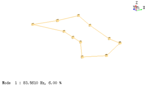
Fig 4 Front sub-frame first order modal test results 83.6Hz
